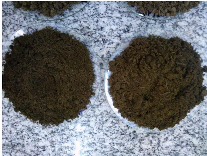
Figure 02: Hydrochar dried in an oven at 60 °C.
